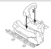
Figure 46 - Installing Log No. 3
